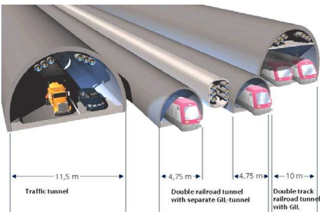
Fig. 7: Typical traffic tunnels for railroad and vehicles
