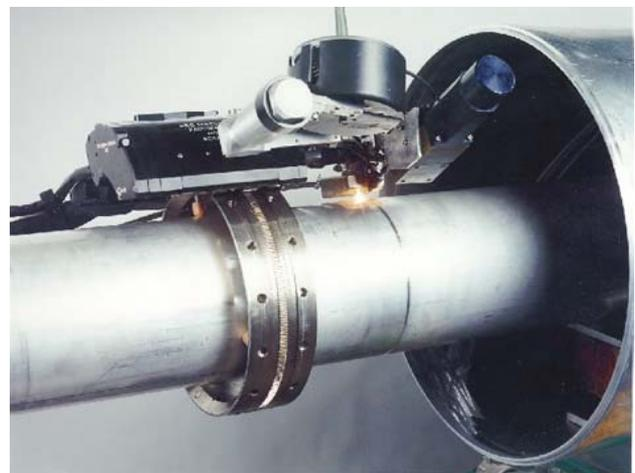
Fig. 2: Orbital welding of the conductor
