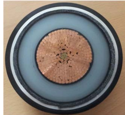
Fig 1. Cables with smooth welded aluminium sheath
