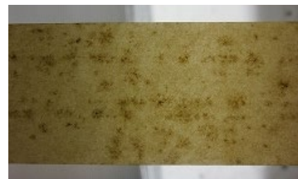
Fig. 2 Black compound on insulation paper
