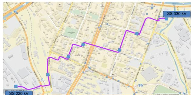
Fig.1. Scheme of laying of cable lines in St. Petersburg.
