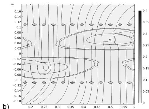
Fig. 2: Geometry of the 3D magnetic flux in the air gap between the conductors, a) x-y cut; b) x-z cut
