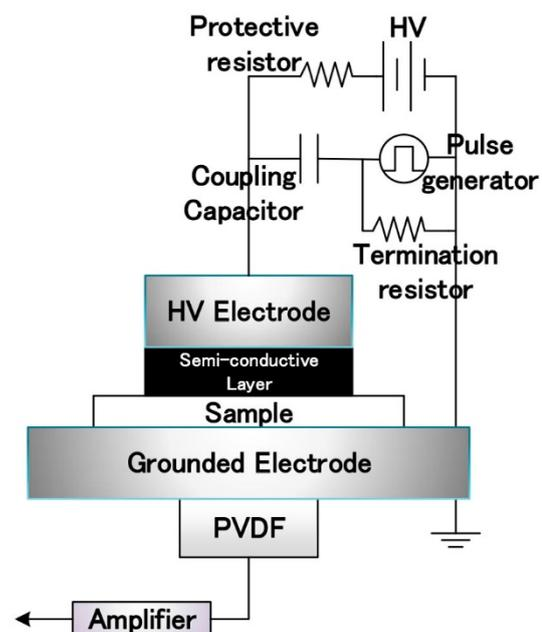
Fig.1 Schematic diagram of PEA measurement system
