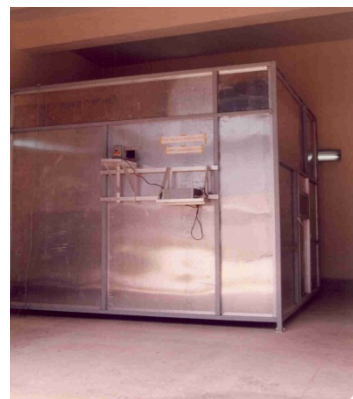
Fig 1. Three metre cube Smoke Test apparatus
