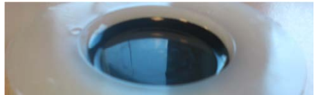
Fig. 1: XLPE sample with semi-conductive electrodes.
