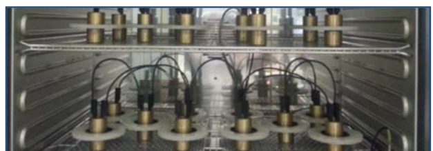
Fig. 2: Ageing test set-up with 0.5 mm samples (up) and 1 mm samples (down).
