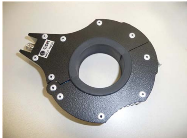
Fig. 1: HFCT used for the measurement
