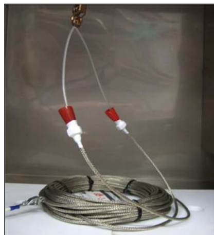
Fig. 1 : Miniature cable with the custom terminations
