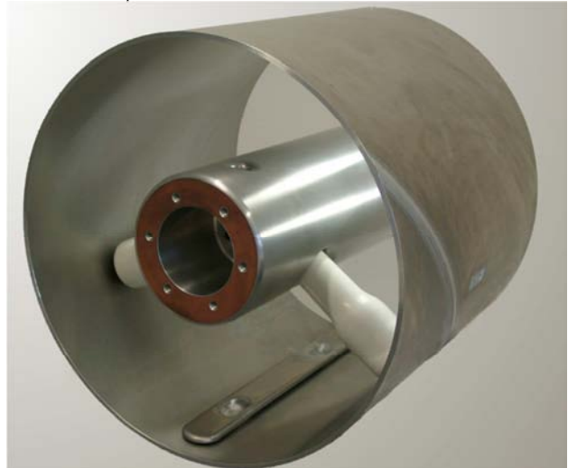
Fig. 1: Basic design of GIL, consisting of two concentric aluminum tubes and cast resin insulators.
