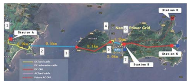
Fig.1: Nan-ao VSC-HVDC pilot project configuration
