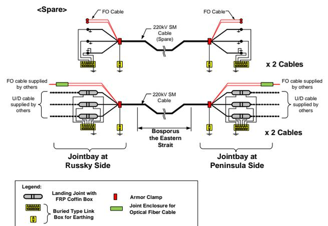
Fig.1: Line diagram of 220kV XLPE submarine cable
