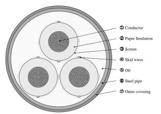
Pipe-type cables are designed with a paper insulated 805mm<sup>2</sup> copper conductor. Three phases are laid in a steel pipe under a 15 bar external pressure.
