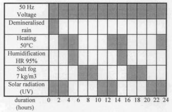
Fig. 1 : Ageing test according IEC 1109.
