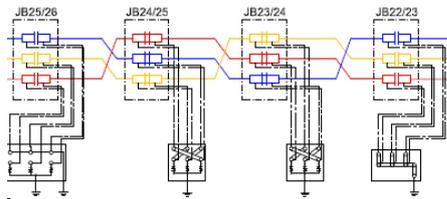
**Figure 5 – Cable cross bonding over 3 sections**
