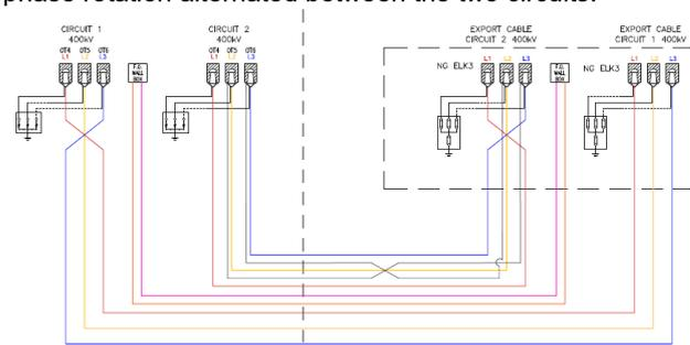
**Figure 9 - 400kV Cable Circuit Configurations**
