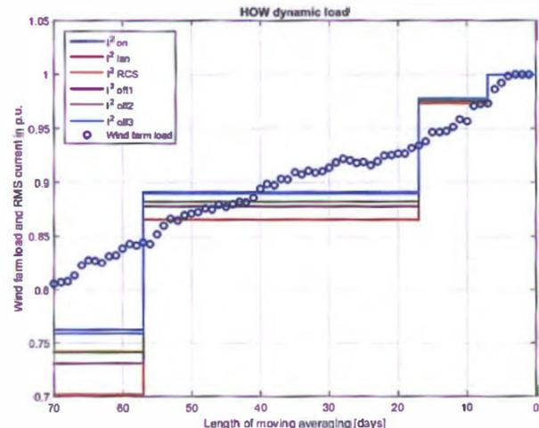
**Figure 10 - Dynamic loading profile for different locations (and thus capacitive current)**
