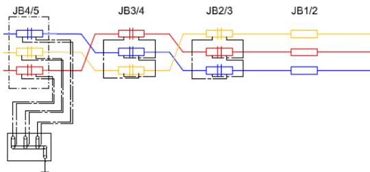
**Figure 7 - Cable Direct Cross Bonded 4 cable sections**
