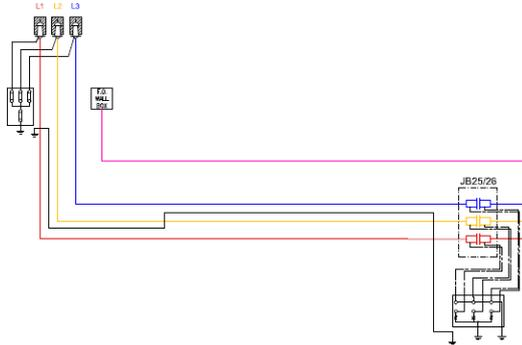
**Figure 4 - Cable end point bonding**
