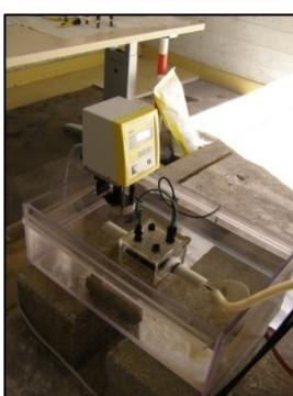
Figure 4: cable sample in salt water during testing
