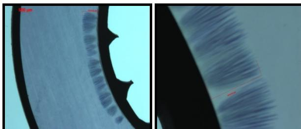
Figure 18: new cable with huge WTs after the accelerated ageing test
