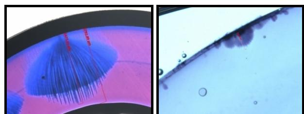
**Figure 13:** vented trees obtained in an aged cable sample before the accelerated test and on another sample after the test
