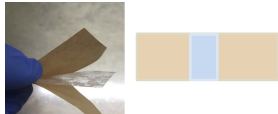
Fig.1: The structure of PPLP with two Kraft paper and one PP layer.
