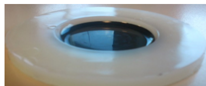
Fig. 1. XLPE Rogowski sample with semi-conductive
