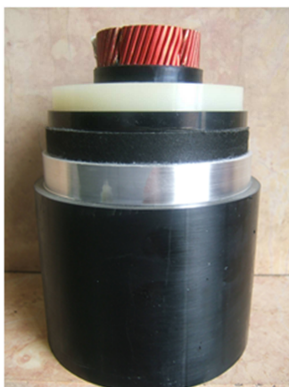
Fig. 7: 2500mm 2 enamelled copper 225 kV XLPE Cable
