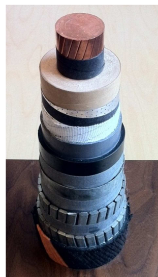
Fig.10: 750 mm 2 Cu +/- 250 kV Mass Impregnated cable
