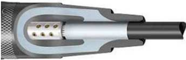
Figure 6. Sketch of deflector shields, grey material layers, made out of conductive rubber in a HV cable joint. The joint insulation material is sketched in blue, the cable insulation in white, and the cable ground layer in black color.
