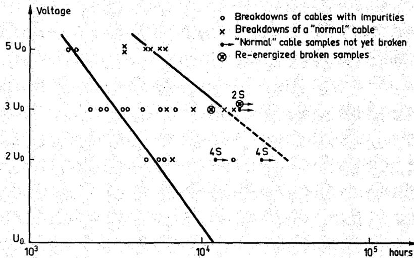
Figure 5c-10. Life durations versus testing voltage of 20-kV cables, the conductors of which are filled with water.
