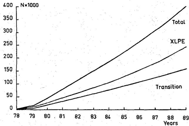
Figure 5c-18. Quantity of HN 33\_S\_23 cable, terminations and joints in service by year.
