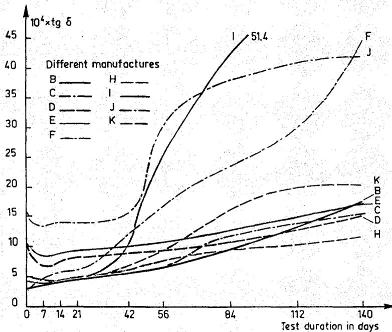
Figure 5c-5. Variation of dielectric loss tangent of XLPE with time at 135°C for a variety of samples from different manufacturers.
