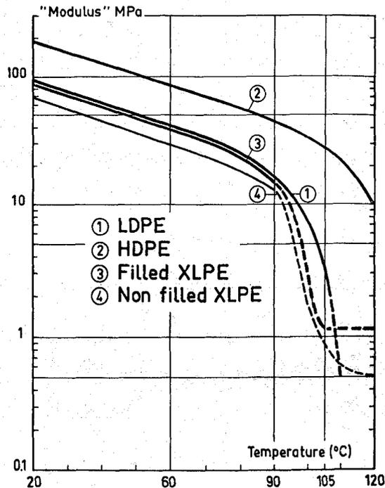
Figure 5c-13. The modulus of four types of polyethylene as a function of temperature.
