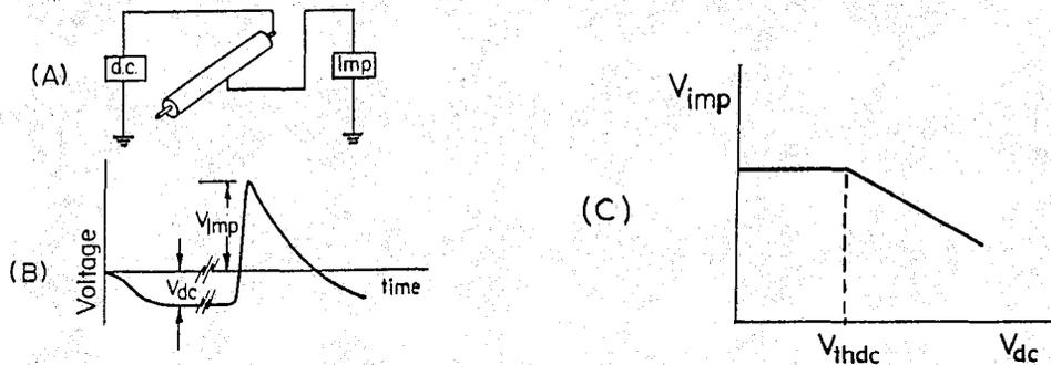
Figure 5e-2. (A) Diagram of circuit for determining threshold voltage. (B) Typical voltage transient. (C) Typical impulse breakdown voltage vs. dc prestressing voltage to establish threshold voltage.
