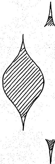
Figure 5b-6. A partially water-filled void in a polymer showing gas trapped in the tip of the void.
