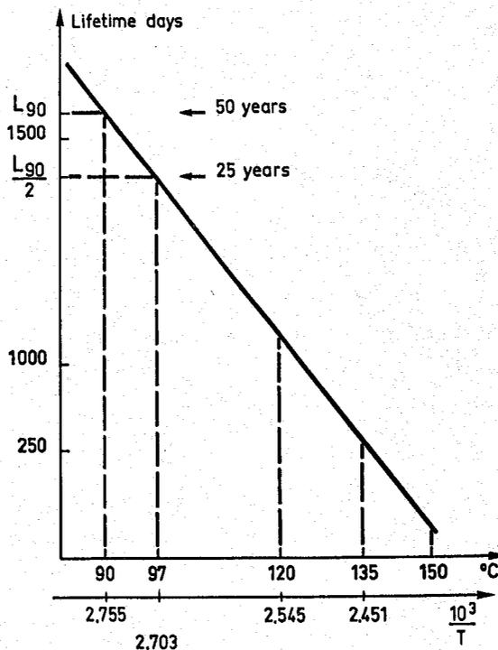
Figure 5c-1. Lifetime for thermal aging of XLPE at various temperatures. This data gives  $A = 11.47$ ,  $E/k = 5730$  for the constants in Eq. 5c-1.
