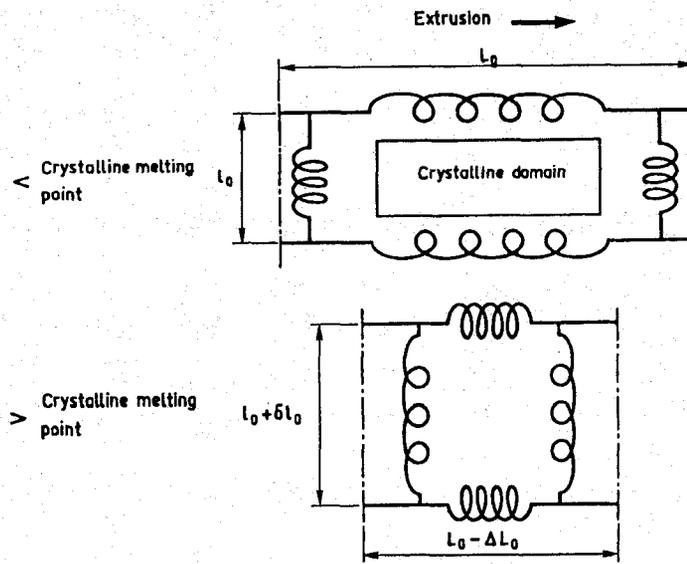
Figure 5c-14. Spring model showing how crystallite melting affects the dimensional changes in polyethylene.
