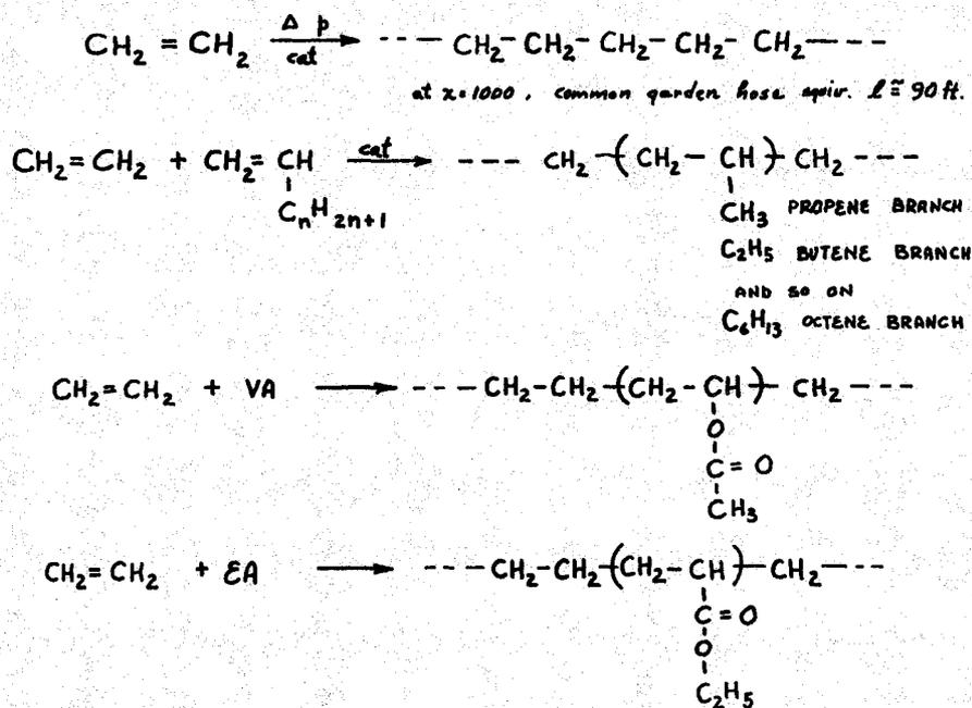
Figure 5b-3. Chemical structures and polymerization reactions of a few common resins that are important to polymer insulated power cables.
