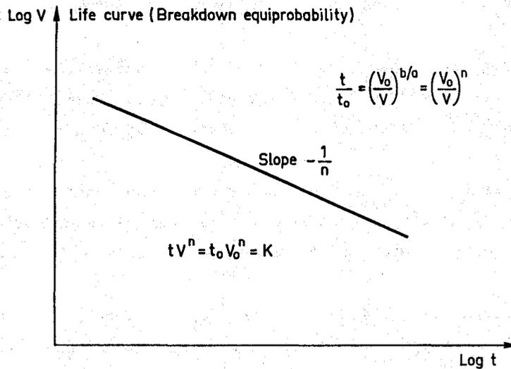
Figure 5c-8. Plot of the life curve given by Eq. 5c-3.
