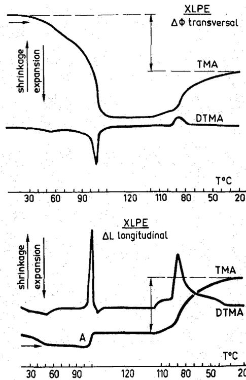
Figure 5c-15. Small-load thermal mechanical and differential mechanical data on XLPE from an extruded cable.
