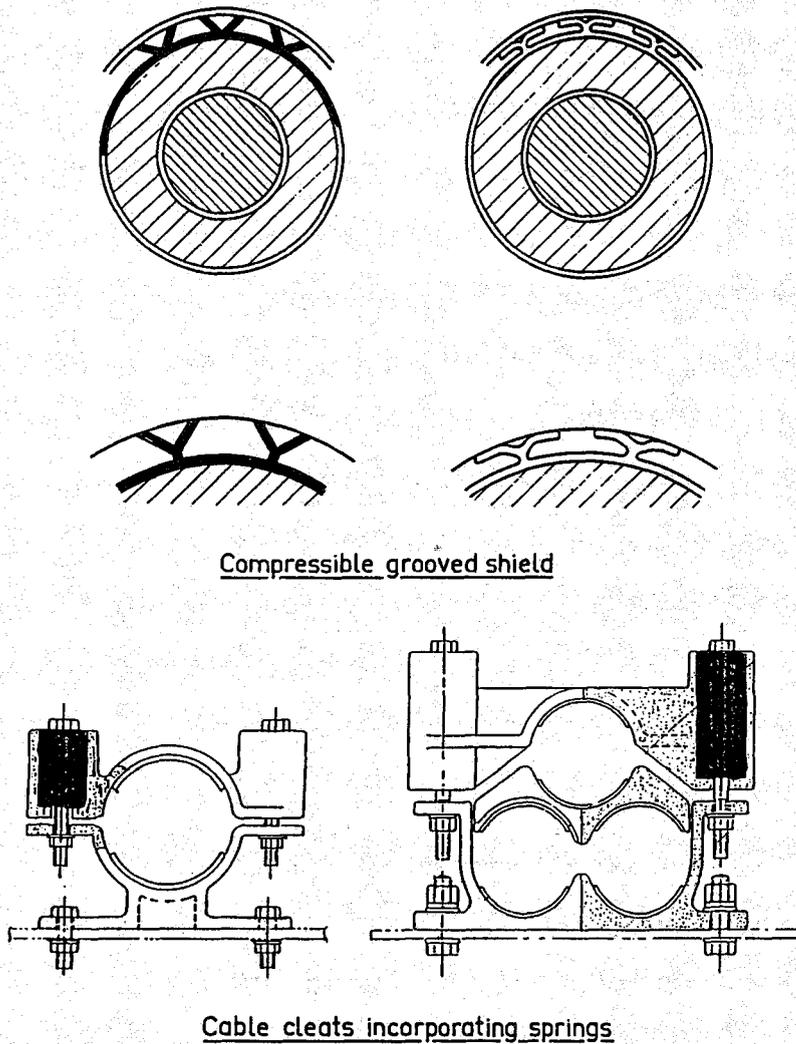
Figure 5c-16. Two designs for relieving thermomechanical stresses in cables.
