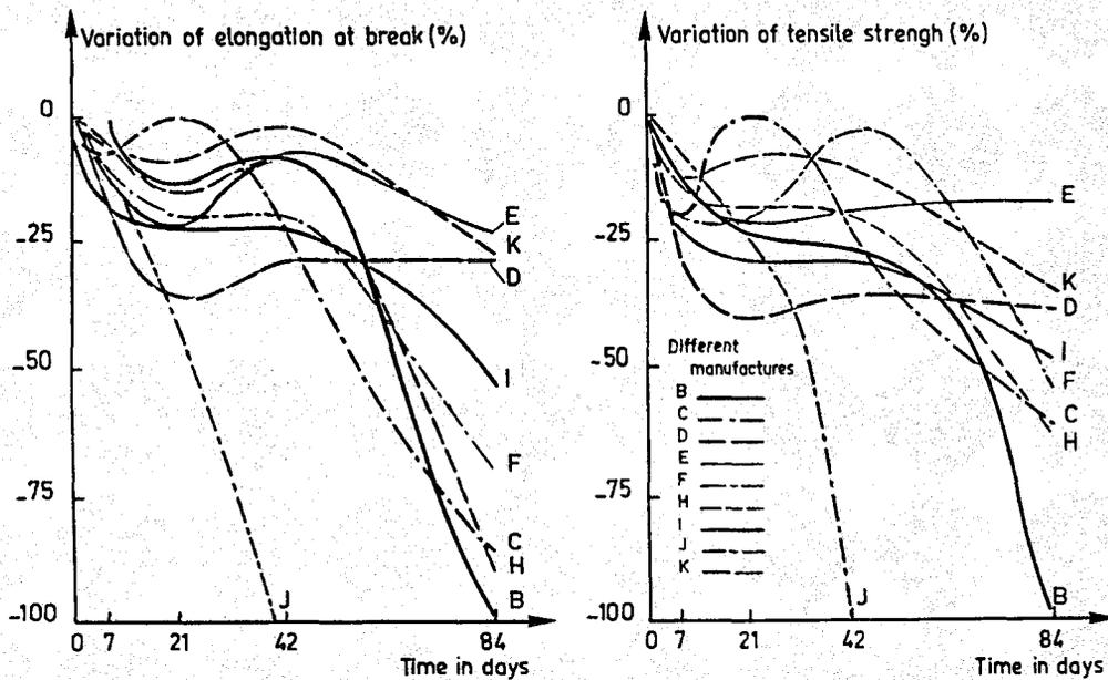
Figure 5c-4. Variation of mechanical properties of XLPE with time at 135°C for a variety of samples from different manufacturers.
