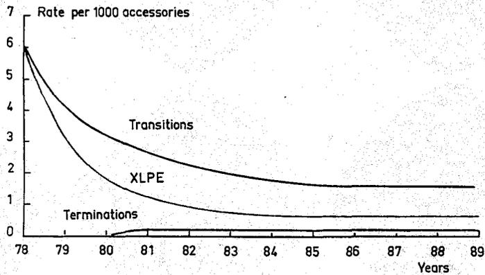
Figure 5c-19. Failure rates for HN\_S\_23 (3 core) cable and accessories by year of service.
