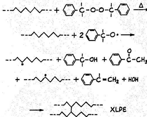
Figure 5b-2. Peroxide crosslinking of polyethylene to make XLPE.
