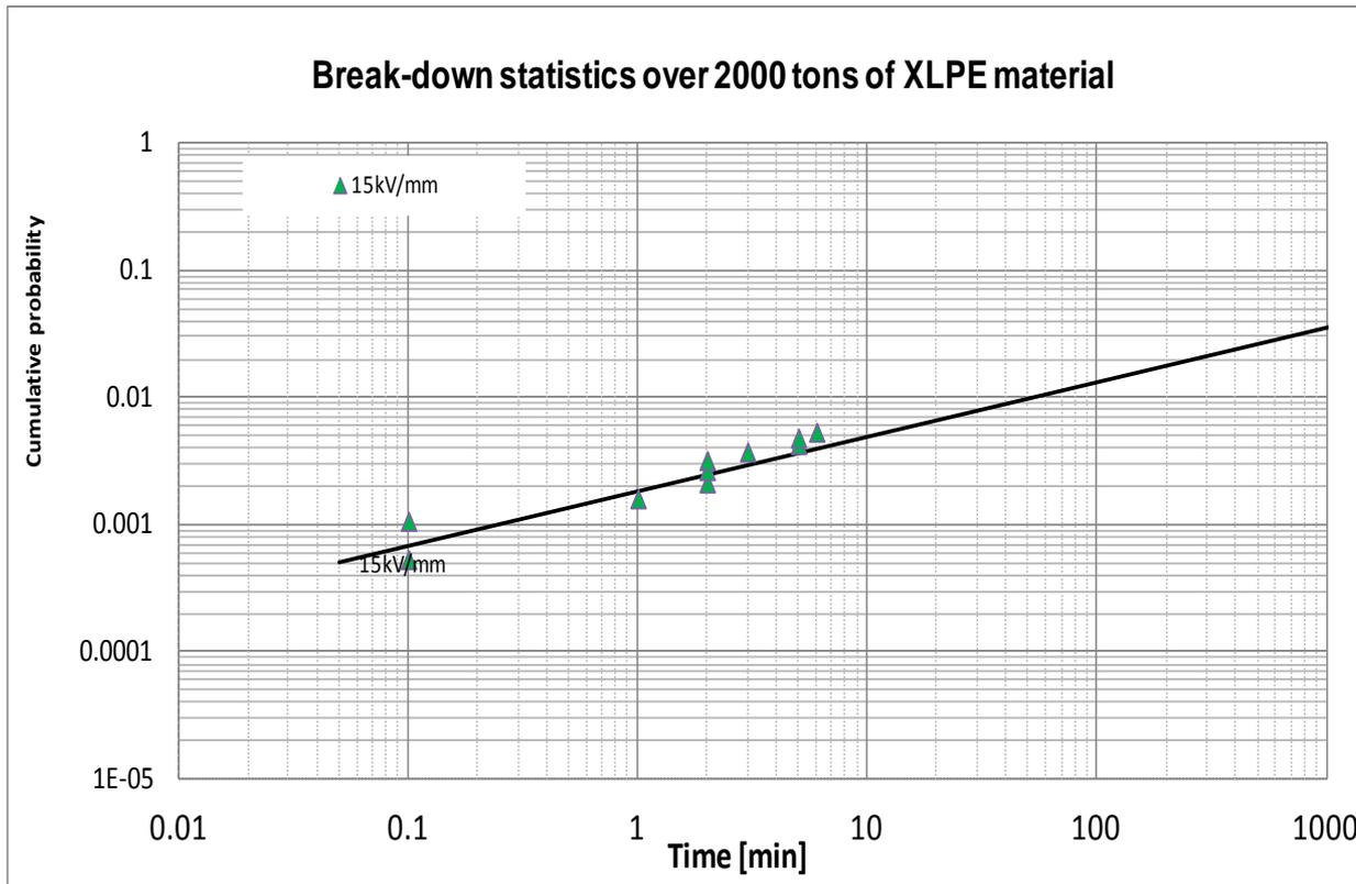
Routine test at 15 kV/mm (4 to 6  $U_0$  depending on insulation thickness).
