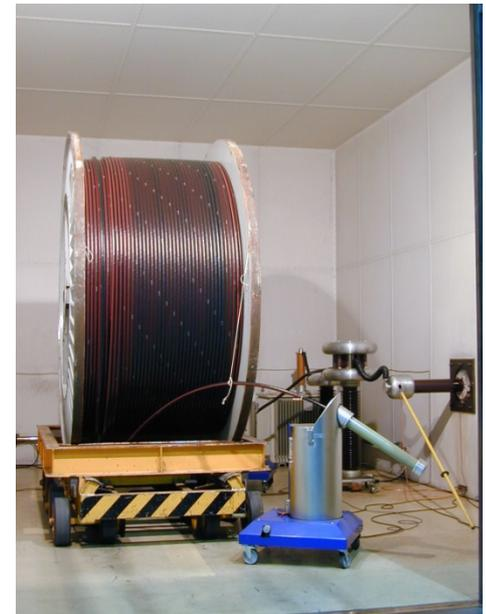
200 tons were tested at 20 kV/mm
