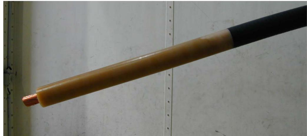
60kV cable with vapour crosslinking:
