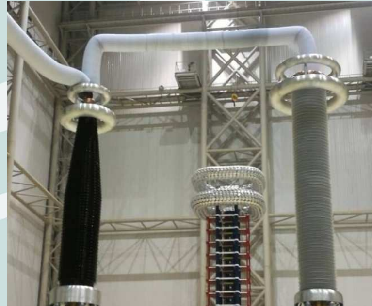
The type test of \pm 500\text{kV} submarine (ChangZhou Test Institution of SGCC)
