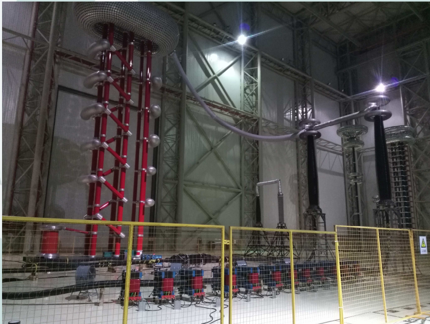
The type test of \pm 500\text{kV} submarine (ChangZhou Test Institution of SGCC)
