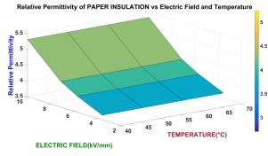
Figure 1: Relative Permittivity of PAPER INSULATION vs. Electric Field and Temperature
