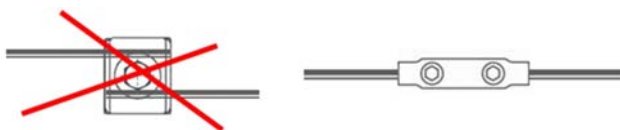
Fig. 1: Connector with and without a necessary overlap of conductors.
