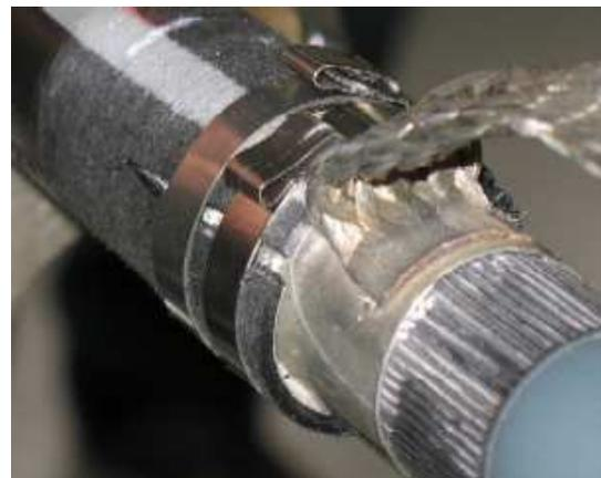
Fig. 3: Screen plate installed on the cable
