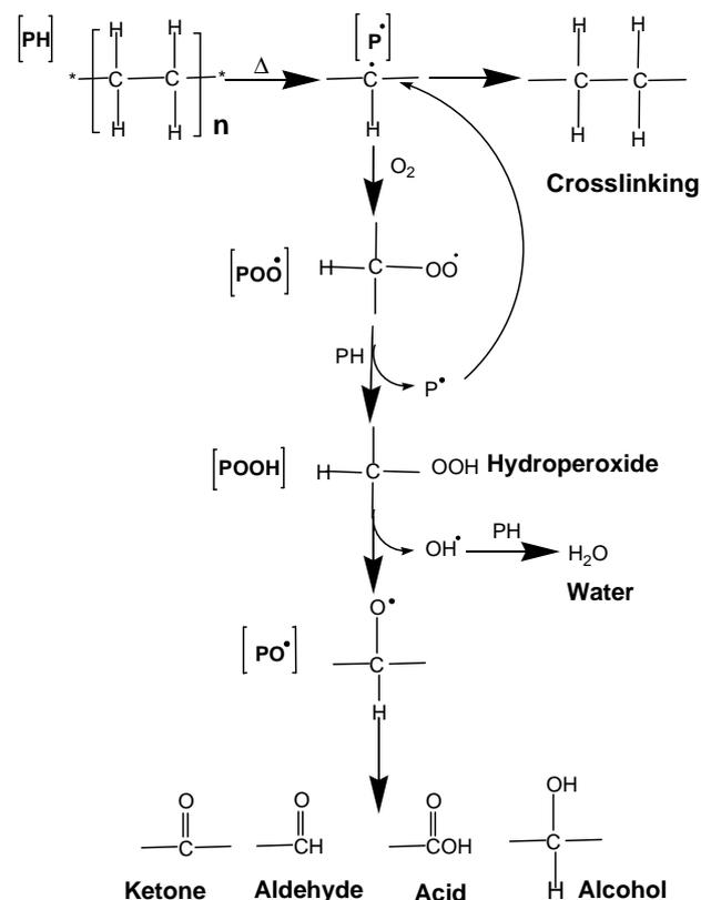
The hydroxyl functions (water, alcohol, hydroperoxide ...) are observed by infrared spectroscopy around 3400 cm<sup>-1</sup> while the carbonyl function appear around 1700 cm<sup>-1</sup>. During these various stages of degradation, the radical (P<sup>•</sup>) dimerises to form a macro polymer (crosslinking) and decomposes by intra and intermolecular reactions to generate Terminal Vinyl bonds ( $\nu = 908 \text{ cm}^{-1}$ ) and Trans Vinyl bonds ( $\nu = 964 \text{ cm}^{-1}$ ) [4-5] (scheme 2).
