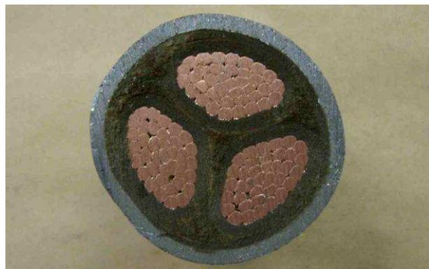
Figure 2 – Cable B: 1940 PILC cable, 66 years service
