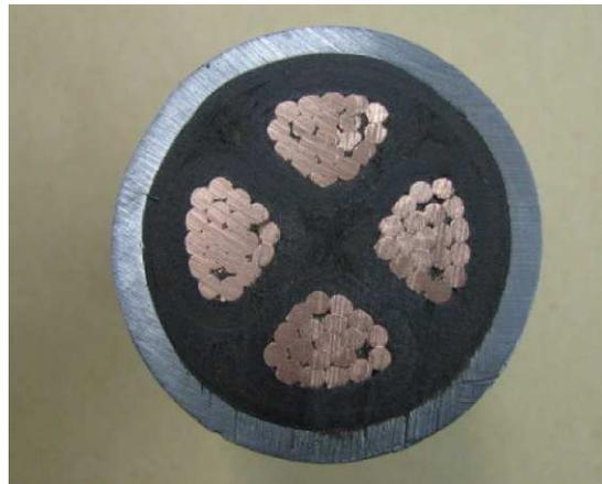
Figure 1 – Cable A: 1937 PILC cable, 68 years service
