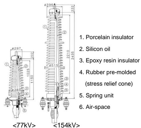
Fig.1: 77/154kV outdoor termination
