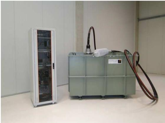
Fig. 1: DRT test system 200kV, 1 $\mu\text{F}$
