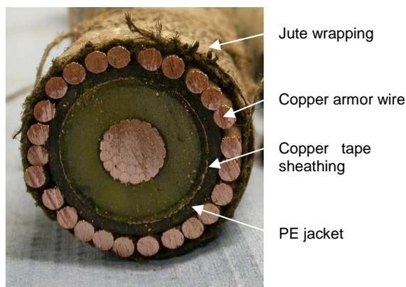
**Fig. 1: Cross-section of the submarine cable**
