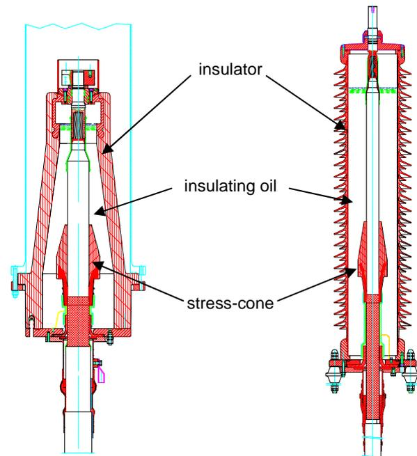
Fig. 1: typical design of fluid filled terminations
