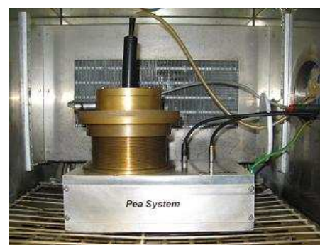
Fig.1: PEA Test bench for plaque specimen up to 30 kV
