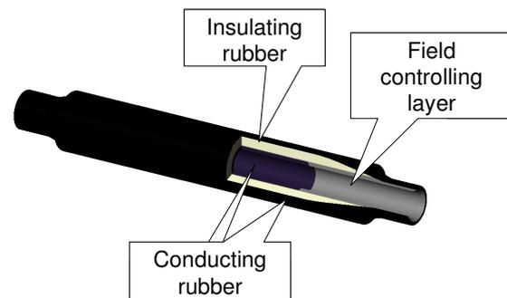
Figure 1. Electrical design of prefabricated joint.
