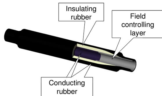
Figure 1. Electrical design of prefabricated joint.
