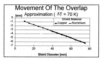
Figure 2: Possible movements of the overlap ( $\Delta T = 70 \text{ K}$ ).
