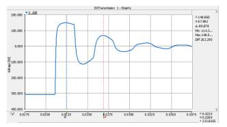
Figure 4 – Example for "oscillating polarity reversals with low frequency" (f  $\approx$  224 Hz)
