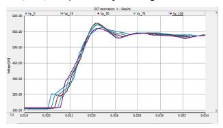
Figure 3 – Voltages at healthy pole during pole to ground fault at different measurement points (0%, 25%, 50%, 75%, 100%) of cable system length
