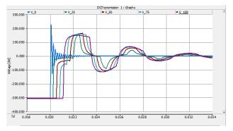
Figure 2 – Voltages at faulted pole during pole to ground fault at different measurement points (0%, 25%, 50%, 75%, 100%) of cable system length
