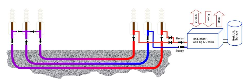
No separate return line required in case of individual cryostats
