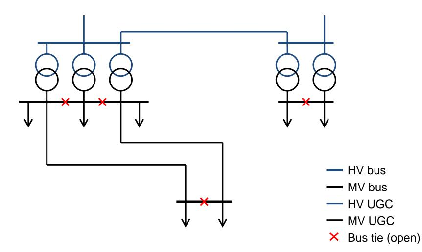
Capacity of one transformer equals total load in each substation
