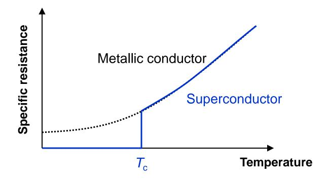
Superconducting state is reached below critical temperature Tc
