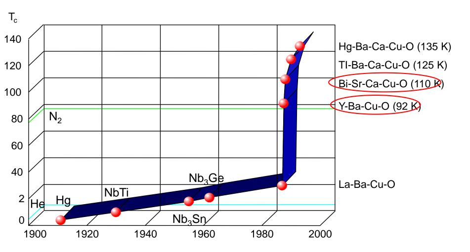
High Temperature Superconductors (HTS) can be cooled with Liquid Nitrogen (LN2)
