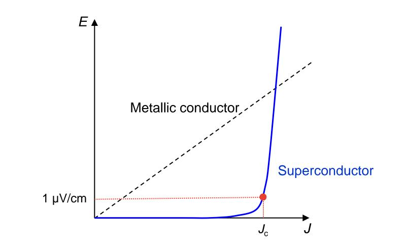
Practical definition of critical current density with 1  $\mu$ V/cm criterion
