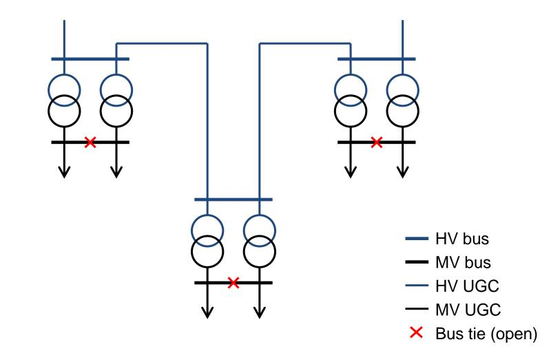
Capacity of one transformer equals total load in each substation
