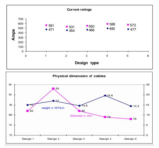
Dimensions and Current ratings of individual construction is as shown in below graphs
