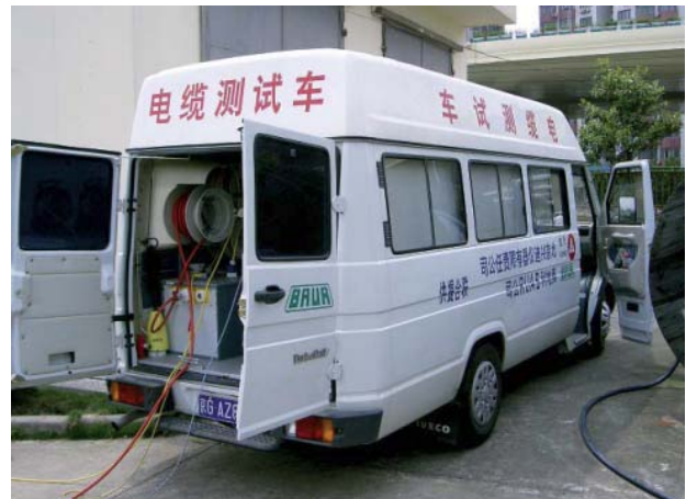
Fig. 11: Cable test vans
