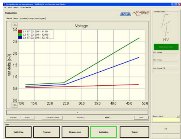
Fig. 6: Results of the \tan \delta measurement in evaluation software
