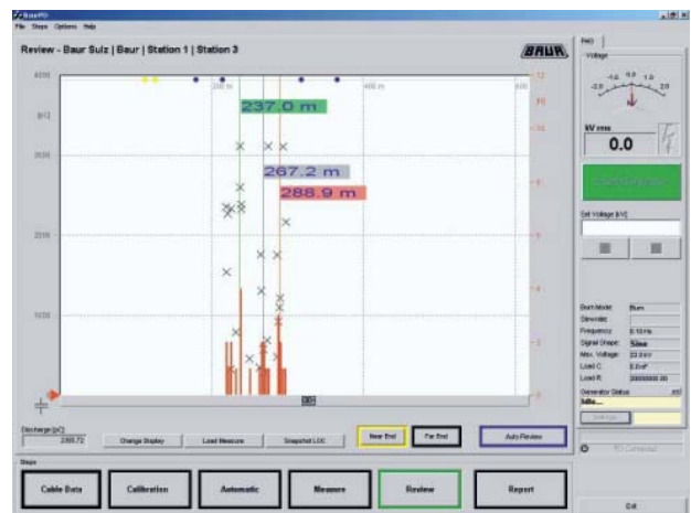
Fig. 8: Faults can be located exactly during the partial discharge measurement on cables
