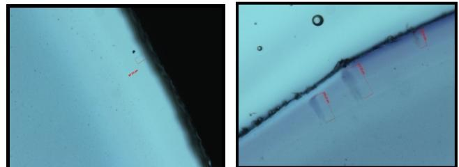
**Figure 12:** vented trees in a cable from 1976 before and after the accelerated ageing test
