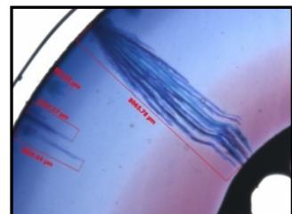
Figure 7: WTs inside the insulation of an aged cable
