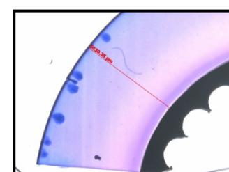
Figure 8: WTs after 7 days in a "homopolymer cable"
