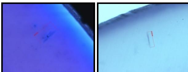
**Figure 14:** bow-tie trees obtained in an aged cable sample before the accelerated test and on another sample after the test
