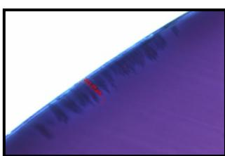
**Figure 9:** WTs after 12 days in a "copolymer cable"
