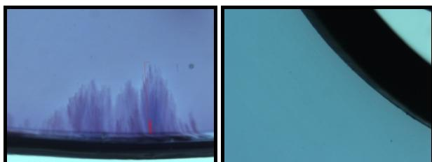
**Figure 15:** cable produced in 1994 and cable produced in 2006 tested with the outer semi-conductive layer
