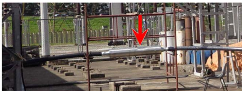
Fig - 2 assembled joint after IEC 60141 tests
