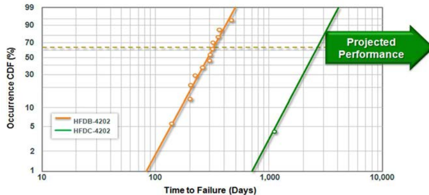
Figure 2: 4,4 ACLT of 15kV medium voltage cable made with C-4202 (4.4mm insulation).
