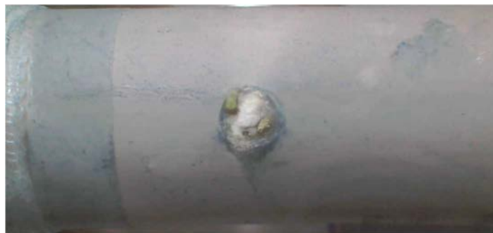
Figure 1: Example of aluminum corrosion in a 6 mm hole.
