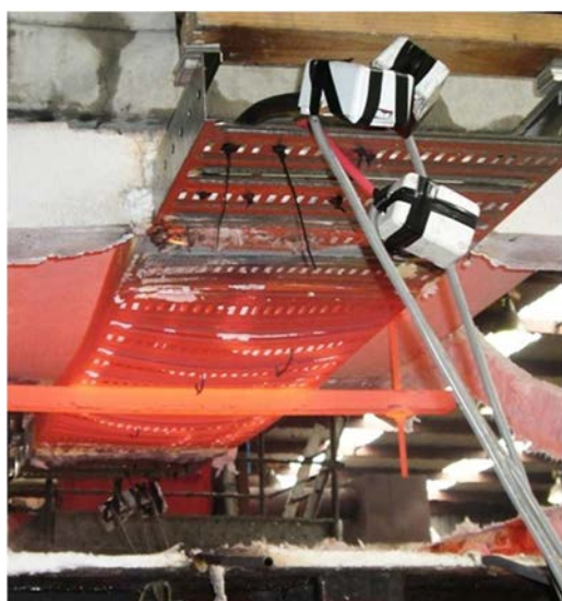
AS/NZS 3013 test conclusion (left); cable residues after the water spray application (right)
