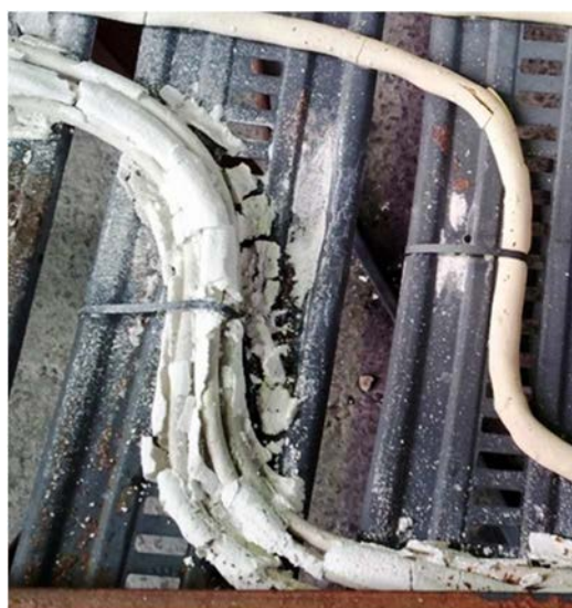
AS/NZS 3013 test conclusion (left); cable residues after the water spray application (right)
