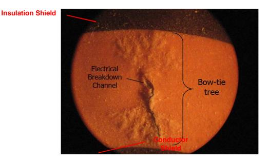
Photomicrograph of the surface of a pink EPR, cross-cut, insulation wafer at the location of AC break down. Bow-tie type water tree spans the whole insulation wall (3.8 mm) from conductor shield to insulation shield.
