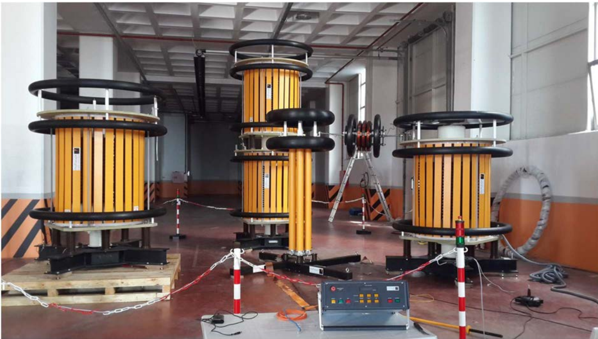
Fig. 1: Frequency Tuned resonant Test System, 350kV, 10A, 10 Hz for On Site Cable Testing
