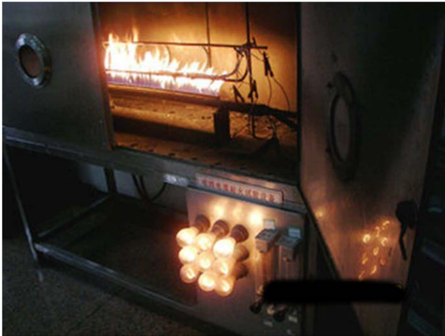
Fig. 1: Picture of a small cable sample undergoing fire testing
