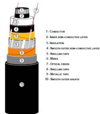
Figure 1: HV cable 110kV with integrated F.O.
