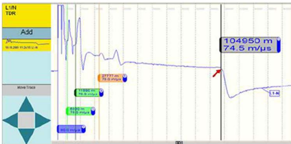
Fig. 1: TDR Trace of a long HVDC submarine cable: SA.CO.I, Italy to Corsica, 105 km
